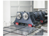
双坐标双主轴结构 Double coordinate double spindle structure
